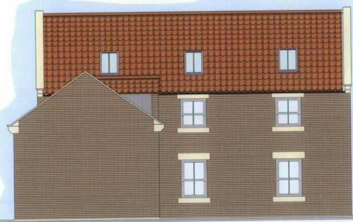
Dwelling Two - Proposed North Elevation ( scale 1:100 )
